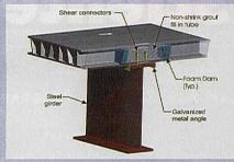
Typical Connection Detail for Steel Girders
