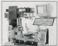
TEACH Lathe and milling in both manual and CNC modes
