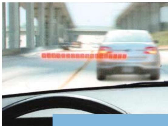
Windshield red alert (above), part of the collision warning system with brake support (at right)
