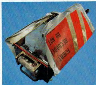
Photo 3 (left)—CVR from a plane that crashed, cut open to access its data
