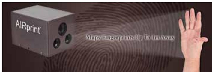
**Photo 1—Each AIRprint unit has two digital cameras, a polarized light source, and the computer power to turn the photos that the cameras take into detailed fingerprint images.**
