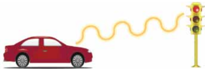
Fig. 3—In car-to-infrastructure communication, a traffic light senses how many cars are waiting on each road that it covers. It can increase traffic flow by keeping its light green where the traffic is greatest on a moment-to-moment basis.
