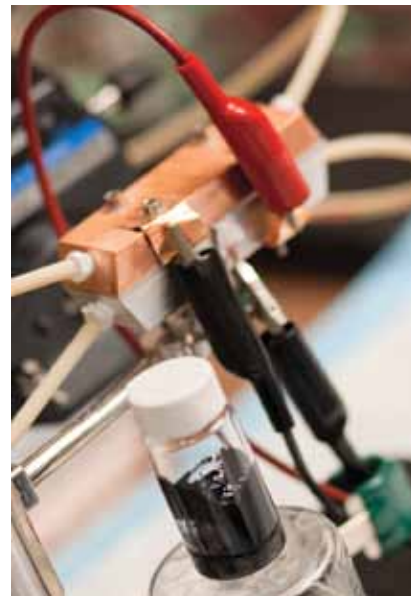
Photo 2—The black liquid in the container is Cambridge Crude. The laboratory bench experiment shown was performed at MIT to serve as a proof of concept that the semi-solid cell battery generates lots of electricity.
