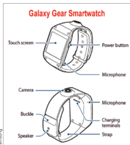
Fig. 1—Details on where Samsung hid the camera and other gear needed for two-way communication on their new smartwatch.
