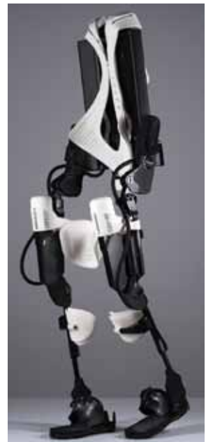
Photo 5—Each exoskeleton is custom made to fit its wearer. The person is 3D scanned; the results become the digital instructions for a 3D printer that generates a perfect-fitting exoskeleton. Motors, sensors, and other actuators are then added so the person can walk again.
