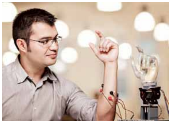
Photo 3—In the same way that strings on a marionette control a puppet's movement, the electrodes on the scientist's arm let his brain control the movement of the cybernetic hand.
