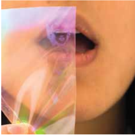
Photo 3—The label shown has an invisible watermark design that will show when you blow moist breath on it.
