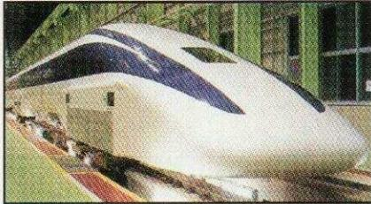
The Japanese are now testing a fully functional 11.5-mile Maglev system. As this system passes operational tests that began in the spring of 1997, the line will be extended so that it eventually connects Osaka and Tokyo. The Japanese Railway Technical Research Institute's Maglev vehicles are designed to travel in a U-shaped guideway with no physical contact with the guideway walls.
