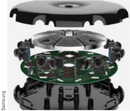
Photo 3—This exploded view shows how Samsung located the equivalent of 16 cameras in their new Project Beyond camera.
