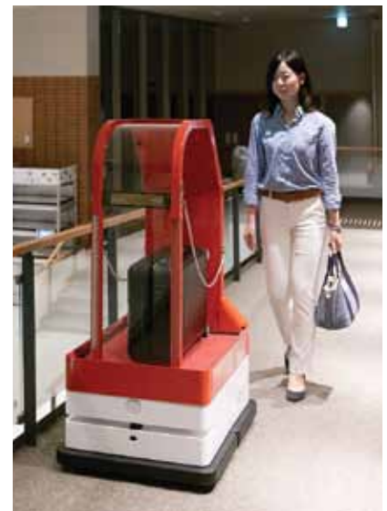
Photo 2—Many of the robots at the hotel have a form that best matches their function. For example, the porter that transports your luggage to your room is a robotic self-driving cart.
