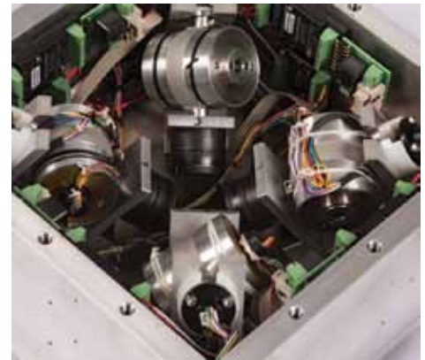
Photo 1—The gyroscopes spin at a constant 15,000 RPMs and the computer rotates them to create the appropriate force.
