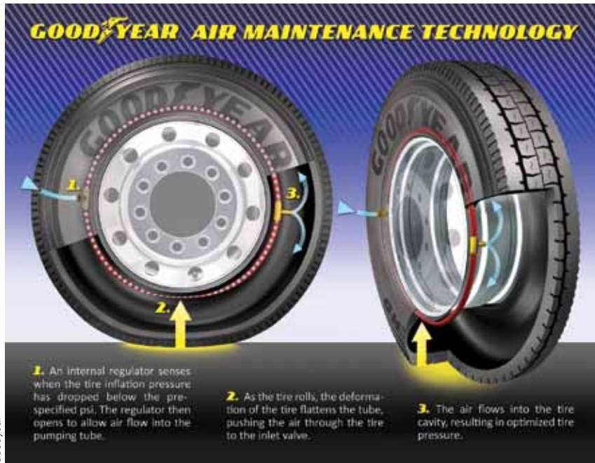
Fig. 1—Operation of Goodyear's self-regulating tire pressure system
