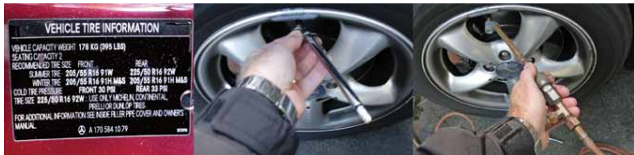
Photo 1—Once a month, you should check to see if all of your tires are properly inflated and follow this procedure: (1) Find your car's tire pressure inflation information; (2) use a tire pressure gauge to determine the current psi for each tire; (3) if a tire is underinflated, pump it up to the proper psi; (4) [not shown] even if the air pump you are using has a pressure gauge, double check that the reading is correct using your own gauge.
