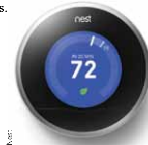
Photo 2 —The Nest Learning Thermostat remembers the temperatures you set and builds its own custom schedule for your home based on what you do.
