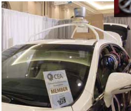
Photo 4—The Velodyne rotating roof laser array, found on Google's self-driving cars, provides the car's electronic vision.
