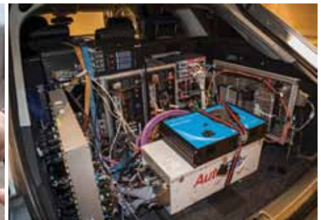
Photo 5—The Audi Connect Piloted Driving vehicle could, under certain driving conditions, take over full control of the car. The equipment to perform this task completely fills the vehicle's trunk.
