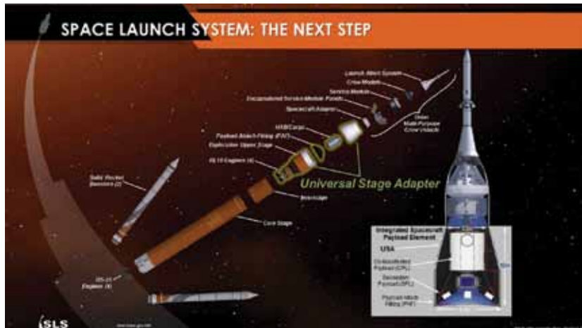
Fig. 1—Size comparison of the parts of the Space Launch System. Note how small the Orion is compared to the hardware that will launch it.
