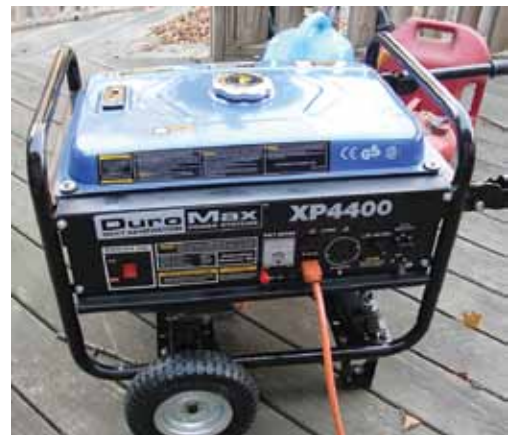
Photo 2—A portable generator can restore some electricity to your home. Generators should always be operated outside and away from windows to keep fumes from entering the home.
