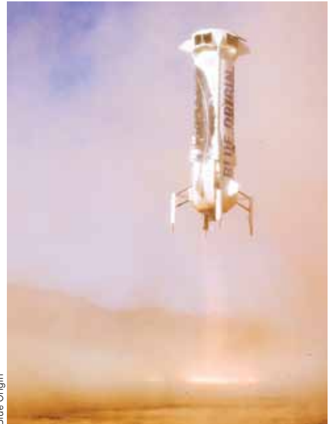
Photo 4 –New Shepard Rocket vertically landing. Its touchdown was at 4.2 mph.
