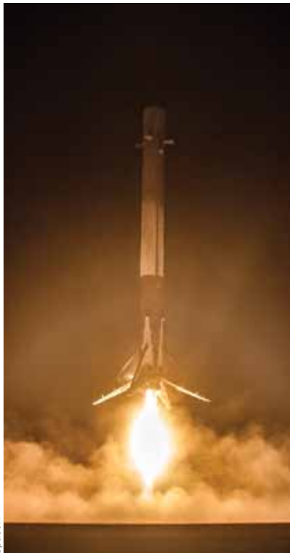
Photo 1—The Falcon 9 moments before it completed its landing. Notice the protruding tripod legs that help stabilize the rocket once it is resting on the ground.
