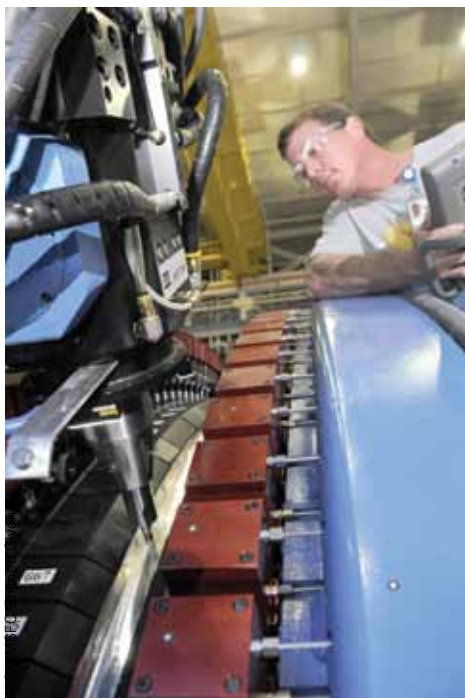
Photo 3— To safely observe this welding process, the technician only needs to wear standard safety glasses.
