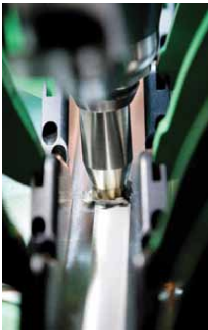
Photo 1—The white line is the section of metal already welded together. The spinning pin tool is pressing against the metal. A computer control system constantly adjusts the tool's rotation speed, travel speed, and surface pressure.
