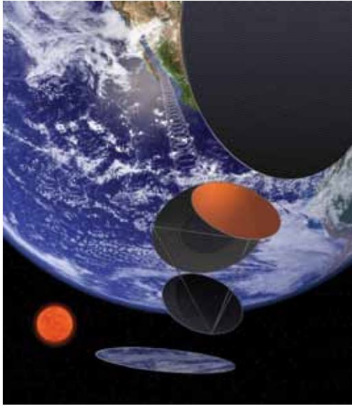
Photo 3—Space mirrors, attached to separate satellites flying in formation with the electricity-generation satellite, would keep the sun fully shining on the photovoltaic panels even at night.
