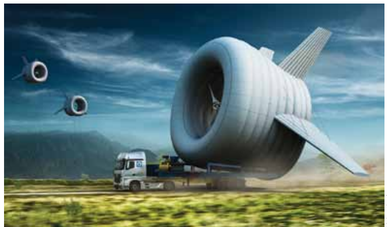
Photo 2—Since its ground station is built physically to fit on a trailer, the BAT can quickly be set up as soon as the trailer reaches the location where it is needed.
