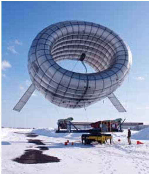
Photo 1—The buoyant air-borne turbine (BAT) is a super-sized wind turbine that floats inside a monster-sized helium donut.
