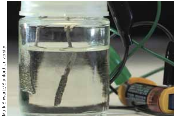
Photo 2—Stanford scientists have developed a low-cost device that uses an ordinary AAA battery to split water into oxygen and hydrogen gas. Gas bubbles are produced by electrodes made of inexpensive nickel and iron.
