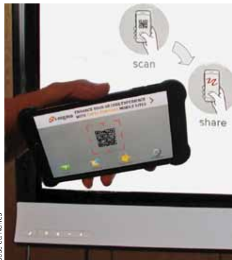
Photo 4—To start a session you capture the QR code at the bottom left of the screen using a QR code reading app on your smartphone or tablet.
