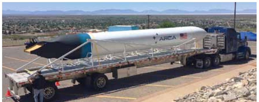
Photo 2—The rocket on the flat bed has the aerospike engine on board, ready to be taken to the launch site. If all goes as planned, it will perform a suborbital space flight. Its sea level thrust will be 4.2 tons from a low-energy propellant. It can reach space because the aerospike engine design lets its nozzle conform to be most efficient for the atmospheric pressure it is flying through.
