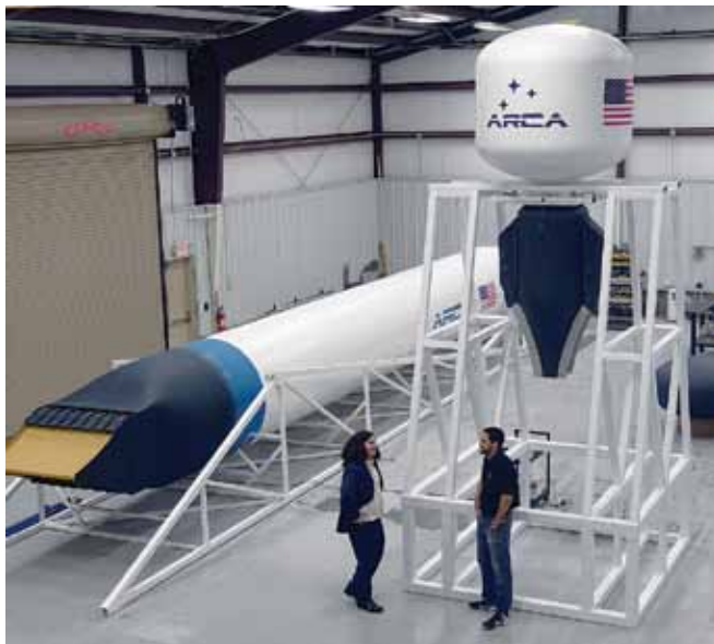
Photo 1—The aerospike demonstrator test engine on the test stand. Within the next few months it should be cleared for a test flight.
