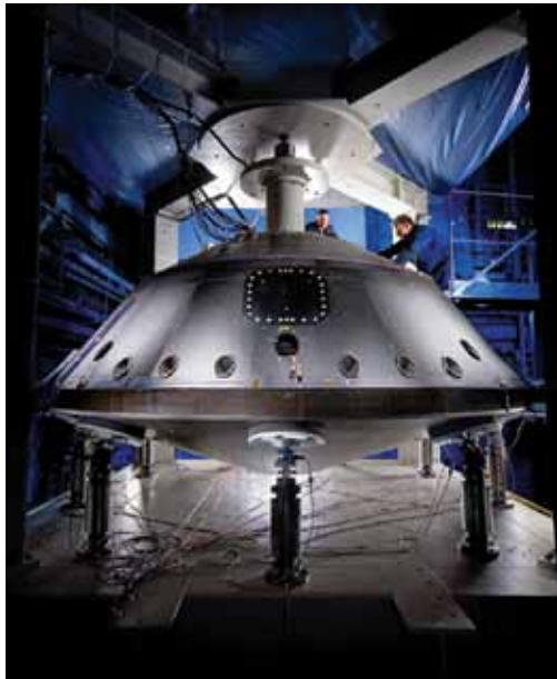
Photo 1— Curiosity 's aeroshell capsule has a back shell and a heat shield. Both parts have the needed thermal protection to survive the heat generated as the rover plummeted through the Martian atmosphere.
