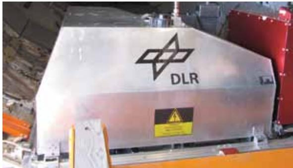
**Photo 4—The DLR Fuel Cell System that was installed on the ATRA experimental aircraft**
