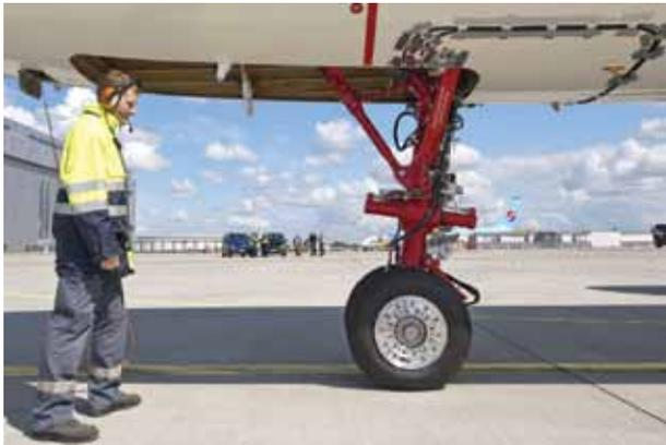
**Photo 3—A test engineer in front of the electric nose wheel**
