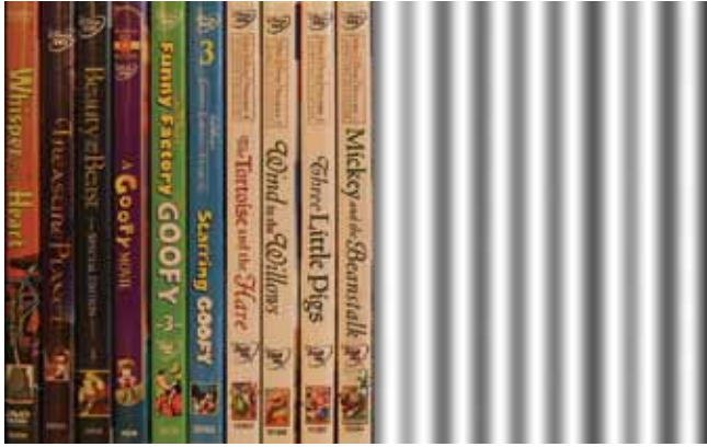
Photo 3 —This photo of a set of DVDs shows the image you see (left side) and a rendering of the tactile disturbances that you would feel (right side) if you were running your fingers across the screen.
