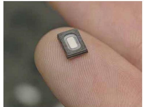
The tiny size of the Micro Mechanical Systems (MEMS) speakers found in the Fauna Glasses.
