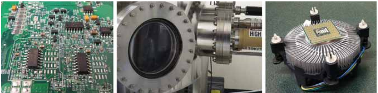
Photo 1—Nano-metallic gluing can attach electronic components without heat, produce a joint that is strong enough to carry loads under pressure, and attach metals to other materials. Its completed joints can conduct electricity.
