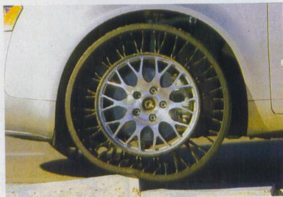
Spokes and tread deform to take the shape of obstacles.
