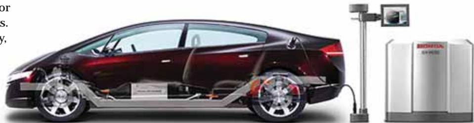
Cutaway view shows fuel-cell components beneath console and rear seat areas.
