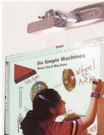
Photo 1— The 3M super-close projection system lets you write on the whiteboard without casting a shadow.
