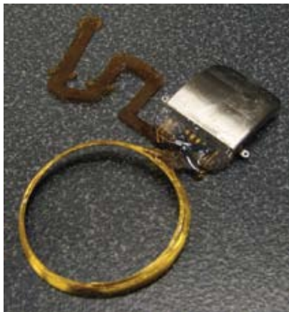
Photo 2 (left)—Receiver coil, microchip, and electrical circuitry are surgically implanted in patient's eye.
