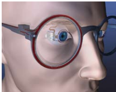
Photo 1—Eyeglass frames transmit video images to the implant's receiver coil.
