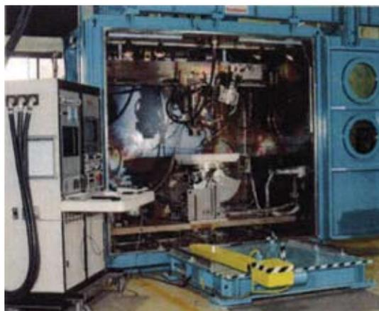
Photo 1— Electron beam free-form fabrication must be performed in a vacuum chamber.
