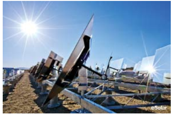
Photo 3—Computers control mirror tilt.
