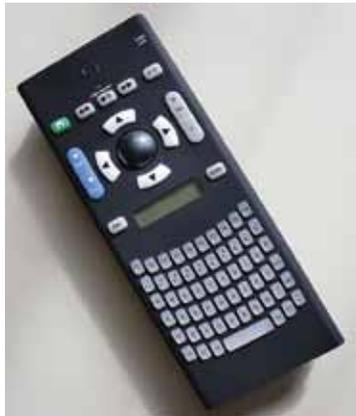
**Photo 4—The IGUGU remote wirelessly controls your computer. To acquire Internet TV, connect your computer to your HDTV with supplied cables or someone else's wireless solution.**
