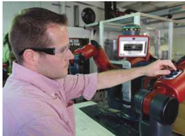
Photo 3—To program Baxter, an instructor grasps its wrist then moves Baxter’s arms and grippers through each movement. Programming is completed using two buttons and one turn knob on Baxter’s arms.
