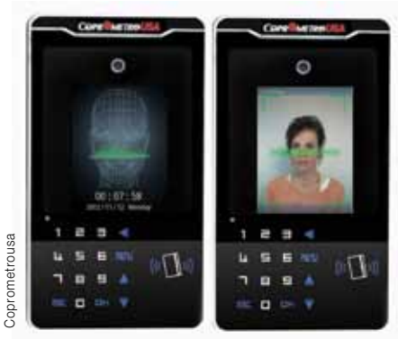
Photo 2—Stone Lock uses a facial biometric authentication system to unlock your door. The system can't be fooled by someone holding up a picture of an approved face.
