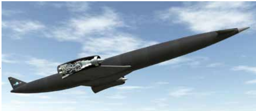
Photo 1—The Skylon spaceship will have two SABRE engines and will be able to fly both as a jet airplane and as a rocket-powered spaceship.
