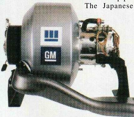
**Photo 2—EV1's gas turbine engine.**
