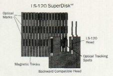
Pig. 2—Optical spots projected through slot in SuperDisk's head.
