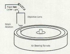
Fig. 1—Laser ablation used to create optical marks on LS120 SuperDisk's surface.
