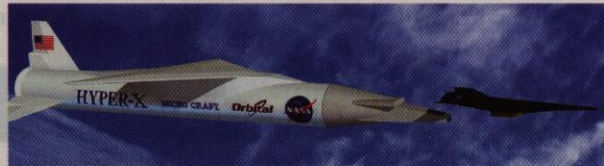
Photo 3—This image, captured from animation video, illustrates the separation of the X-43A from the Pegasus booster.
