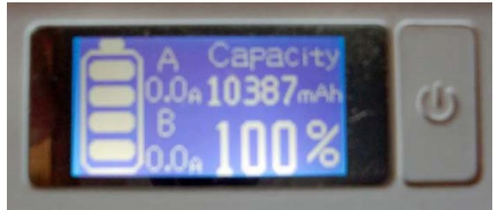
will need to be recharged. The display also shows you how much electricity your device is drawing from the charger during the charging process. See photo 2.
