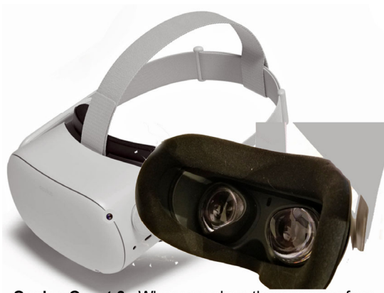
Oculus Quest 2 - When you place them on your face your left and right eye have their own video screen.
