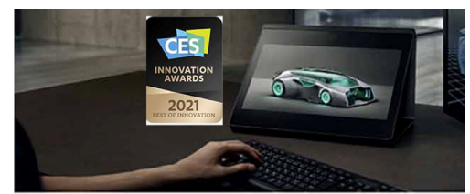
Sony's Spacial Reality Display Micro-optical lenses send separate images to each eye
