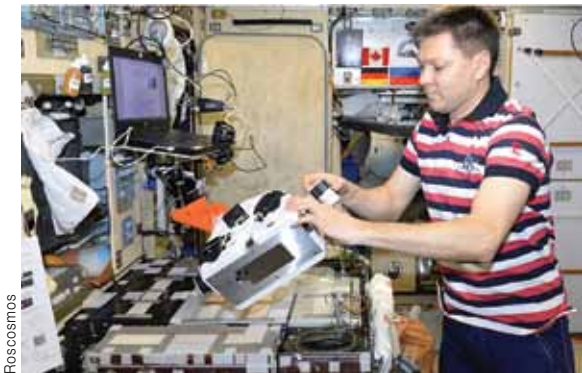
Photo 5 (below) —In zero gravity, this Russian Cosmonaut used a bioprinter to print living human cartilage tissue. Astronauts and Cosmonauts are determining the feasibility of using 3D printers to produce what is needed to fix the craft and crew during deep space missions.
