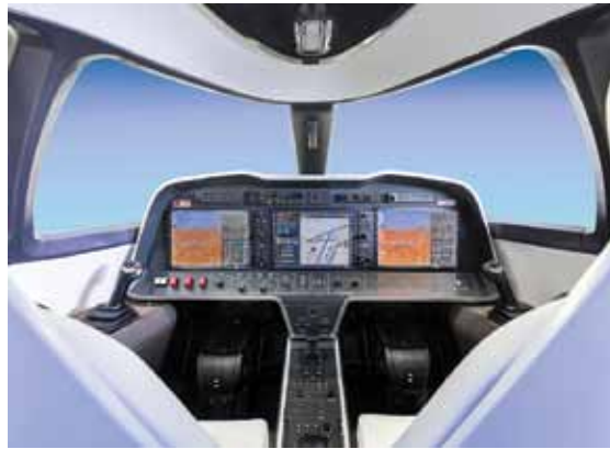
Photo 3—Alice has the newest fly-by-wire technology so its autopilot can handle a flight from takeoff to landing.
