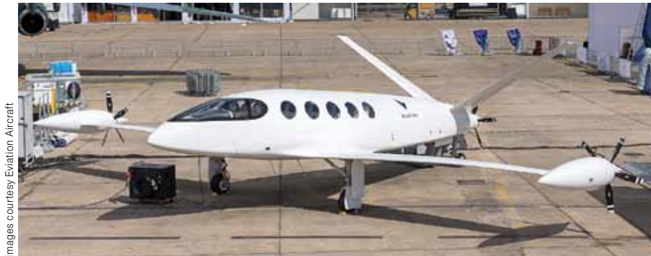
Photo 1—The Alice aircraft is powered only by its lithium ion batteries.
