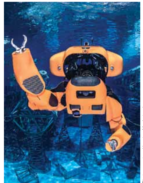
Photo 2—When the Aquanaut Transformer shape-shifts, it becomes a very powerful humanoid robot that can perform all kinds of underwater construction tasks.
