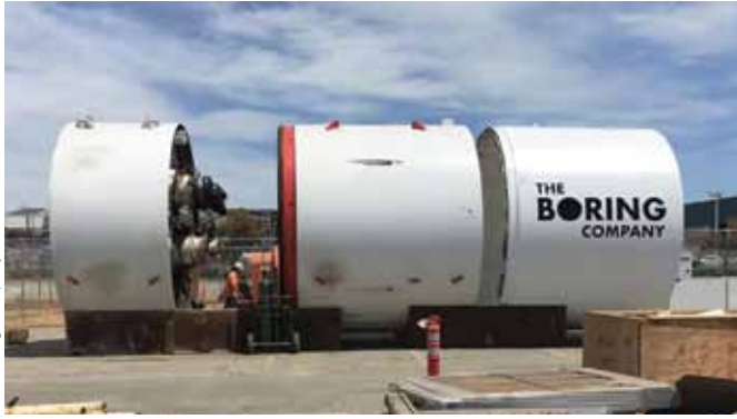
Photo 3— Side view of Godot, the boring machine that Musk's engineers have created.
