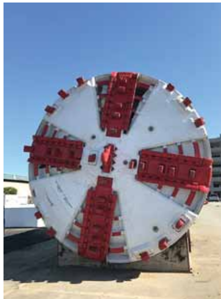
Photo 4 —Cutting end of Godot. It can cut through all kinds of rock and soil, and not get bogged down in mud or other impediments that clog other machines.
