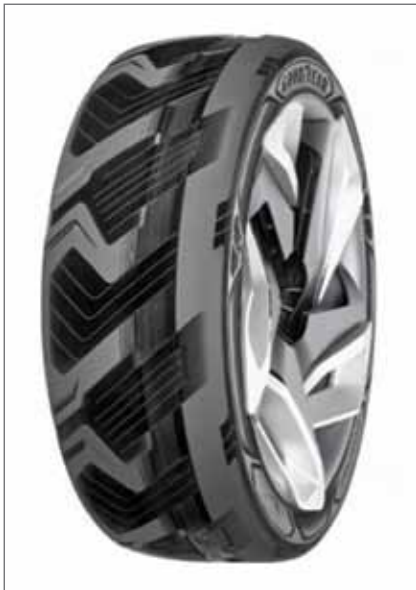
Photo 1—The Goodyear BHO3 is a prototype car tire that generates electricity.
